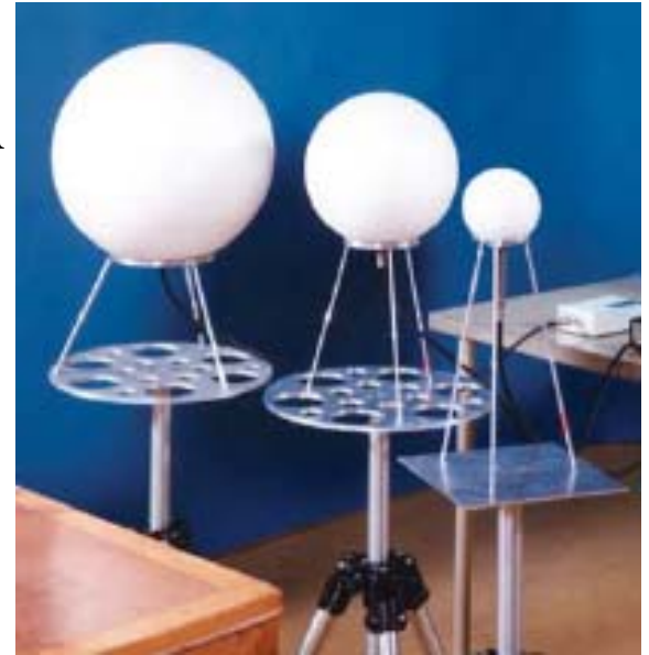
Bonner spheres for neutron moderation
