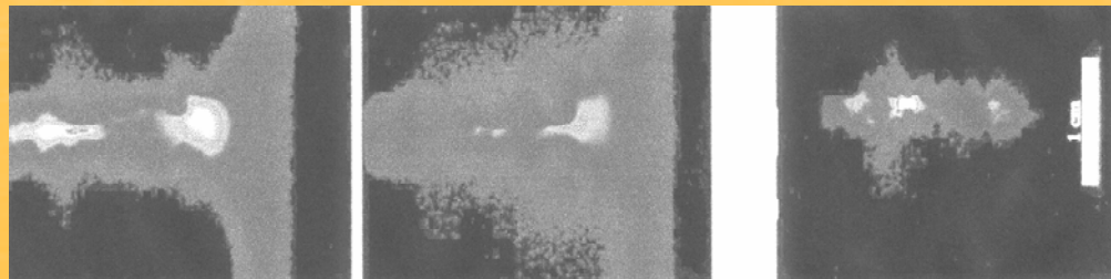
Hot-spots in PF-360 discharges. VR pictures (left) were taken with 1-ns exposition, at 31 ns and 41 ns after the maximum pinch, and the X-ray image (right) - at 28 ns.
