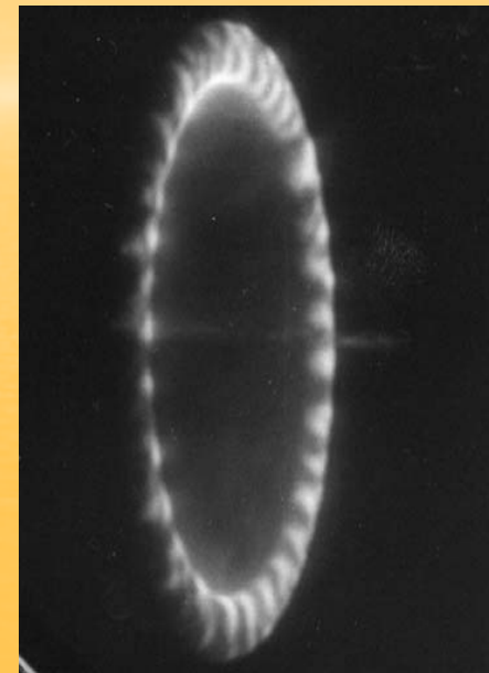
X-ray pinhole picture from another shot, which show very distinct spots of current filaments on the electrode edge.
